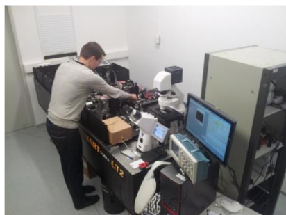
Custom two-channel STED microscope based on Zeiss Axio-Observer and Fianium super-continuum laser
